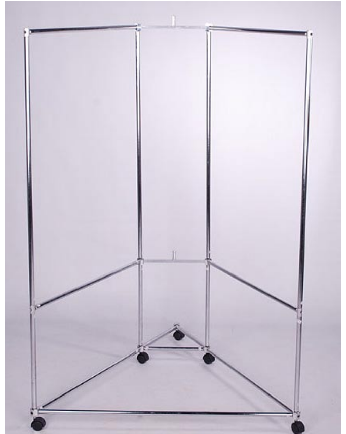
Step 6 – Base with layers A and B attached. A and B contain the light mounts
